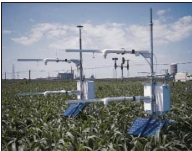
Bowen Ratio Systems calculate evapotranspiration and CO 2 fluxes over a sorghum field near Lincoln, Nebraska.
