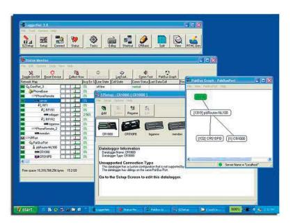
Besides supporting communications between one datalogger and a PC, LoggerNet can manage small and large datalogger networks.
